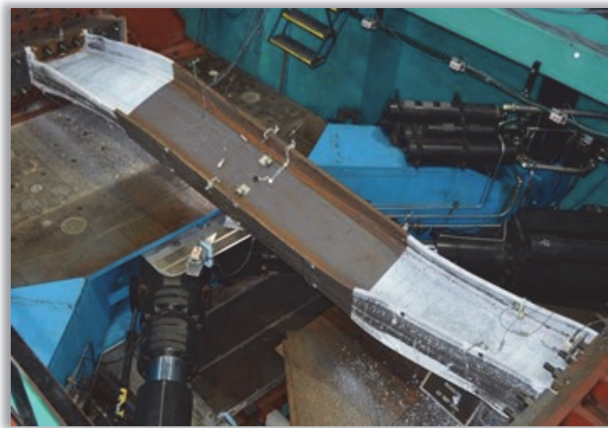
Figure 2-6. Seismic response test of a deep, slender wide-flange structural steel column at the University of California, San Diego (UCSD) with the CALTRANS Seismic Response Modification Device. The columns are commonly used in steel-frame buildings. This research project was a collaboration between NIST, American Institute of Steel Construction, Applied Technology Council, and UCSD. Photo courtesy of C.-M. Uang at UCSD.
